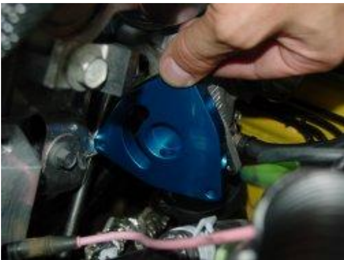
Figure 5 Be sure to align the Converter Plate correctly, the half-moon shape is toward the passenger side of the vehicle, the center hole is toward the front of the vehicle.
