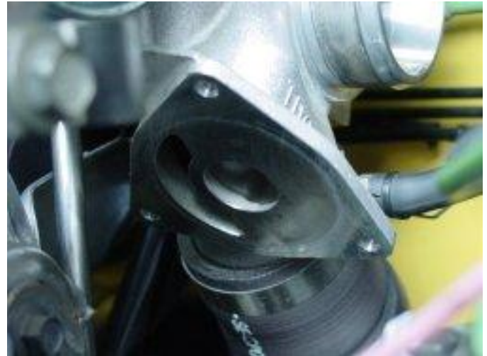
Figure 4 The BOV and internal diaphragm are both removed. Notice how the diaphragm sits inside the BOV. The diaphragm does not have a 'top' or 'bottom', but it does have a 'front' and 'back'.
