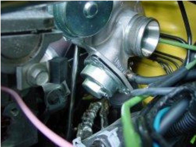
Figure 3 Remove the Pink Vacuum Line and three 10mm bolts that secure the BOV to the turbo housing. The bolt that is not visible in the photo is the tough one. The steel oil line that passes in front of the bolt and connects to the top of the turbocharger needs to be moved. Either disconnect it from the turbo, or carefully bend it toward the exhaust manifold to allow access.
