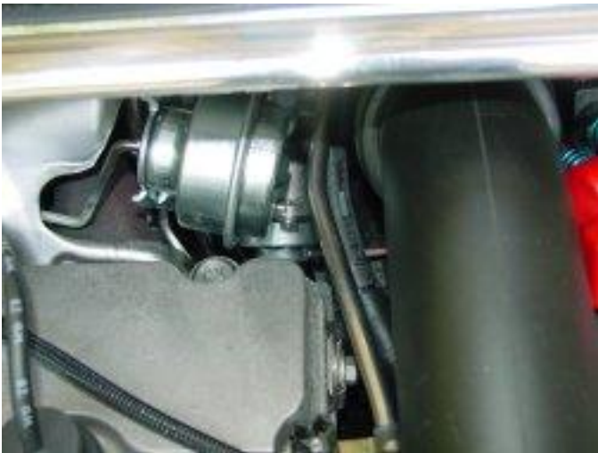
Figure 1 The enclosed instructions advise you to remove the air intake tube and the battery. It’s a good idea, the Blow-Off Valve in there somewhere.
