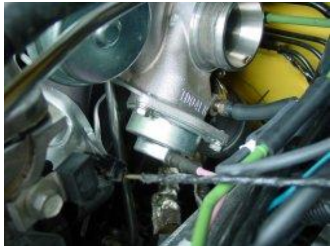
Figure 2 After removing the airbox, intake tube, and battery, the Blow-Off Valve is easy to locate, and service where it is attached to the turbocharger.
