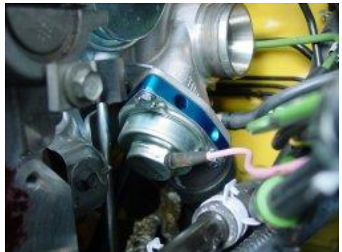
Figure 6 Using the supplied bolts and washers, install the Blow-Off Valve Conversion kit. The Included gasket is sandwiched between the turbo housing and the Converter Plate.
